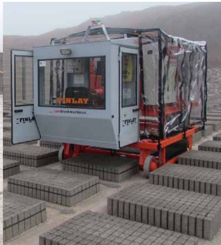
BSM 412 fully refurbished by RPM Block Machines commissioned on site in Scotland.
